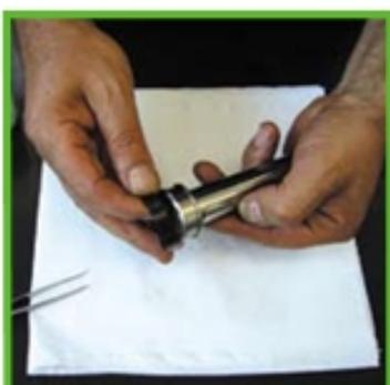
E) Using the special T-shaped tool screwed onto the end of the rod withdraw it with the ferrule. F) Remove the rod from the ferrule.
